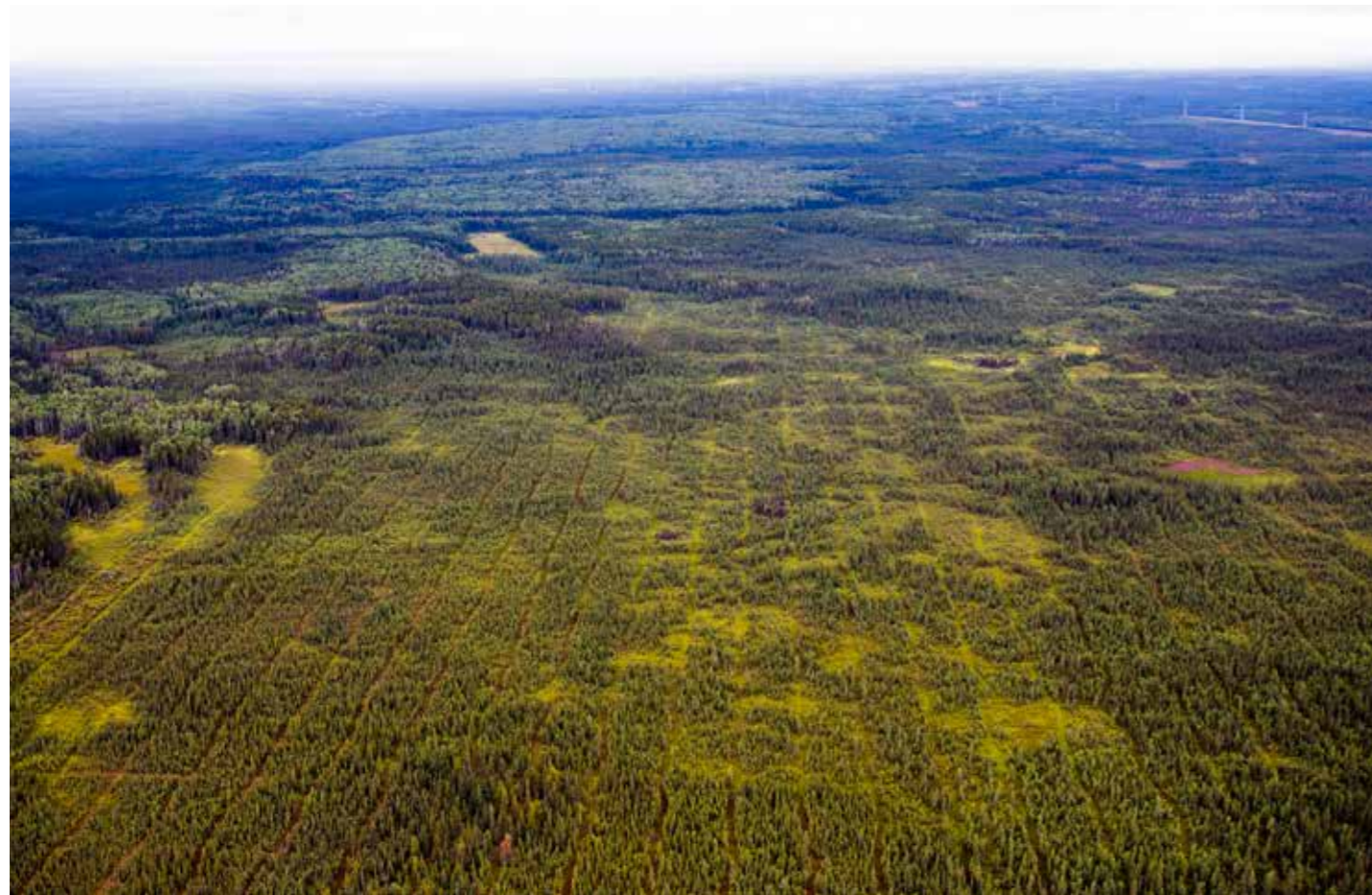
Canada's Bitumen Landscapes - In-Situ Extraction The images on this page show the range of patterns that bitumen exploration leaves behind. Each picture shows seismic cut lines and test well pad sites, but on each site, the pattern is slightly different. (All images Christina Milos 2015)
