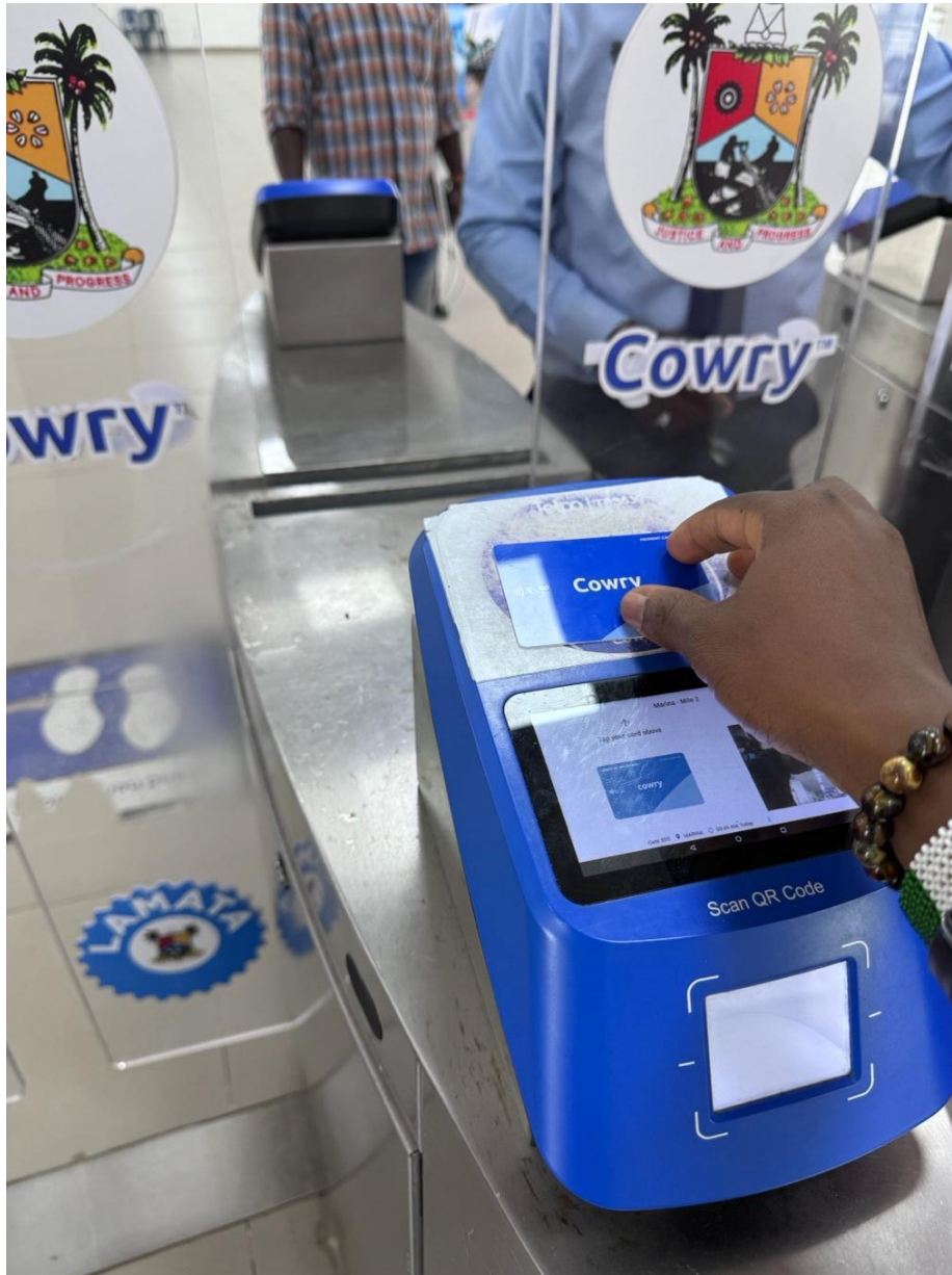
Figure 5. Commuters must touch their Cowry card on the card reader to board the trains and to exit at their destination. Photo credit: Temilade Sesan.
